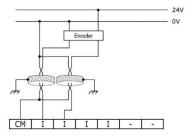
High Speed Input wiring, source
