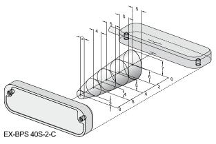
Assured switching distance:  $s_{ao} = 8 \text{ mm}$ Assured switch-off distance:  $s_{ar} = 18 \text{ mm}$
