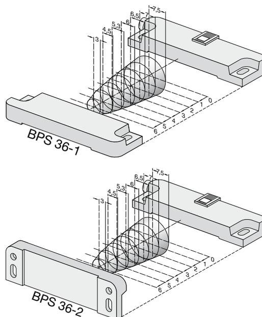
Assured switching distance:  $S_{ao} = 6 \text{ mm}$
