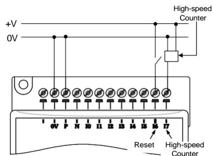
**Wiring the Output's Power Supply**
