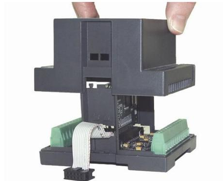
4. The jumpers are shown at right. Change the jumper settings as required, in accordance with the tables shown on the next page.
