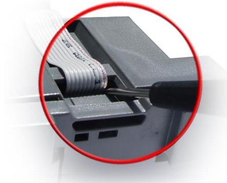
3. Gently remove the top of the device as shown.
