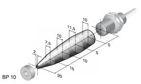
assured switching distance:  $s_{ao} = 10 \text{ mm (BP 6 / BP 8)}$
