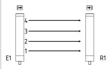
The function of floating blanking is allowed for only one beam taking into consideration the protective function. This function can be used for temporary beam suppression due to environmental conditions. The first beam line, which realises the optical synchronisation and is located immediately behind the diagnostic window, cannot be blanked.
