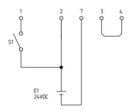
The parameter configuration EDM is activated for at least 2 seconds when the system starts if there is a wire link between OSSD 1  $\rightarrow$  OSSD2 and a +24V level on the input restart interlock.
