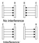
beam coding A required!
