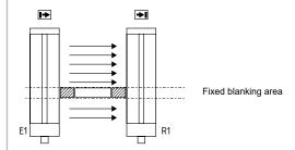
The range of the fixed blanking can be arbitrarily chosen in the protection field.
