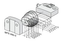
Assured switching distance:  $s_{ao} = 5 \text{ mm}$
