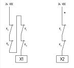
Fig. 7: SRB400CA, SRB400CS and SRB400CA/Q, SRB400SNA left = switch-off level 1 right = switch-off level 2
