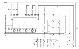
Fig. 2: SRB400CS, SRB400CS/T, SRB400SNA a) Logic
