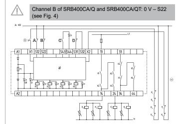
Fig. 3: SRB400CA, SRB400CA/T, SRB400CA/Q, SRB400CA/QT a) Logic
