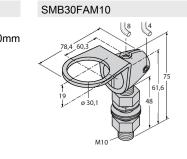
Mounting bracket, stainless steel, for M10 x 1.5 thread, thread length 30  $^{\rm mm}$
