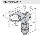
3011185 Mounting bracket, stainless steel, for M10 x 1.5 thread, thread length 30
