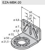
3072587 Mounting bracket, steel, blackfinished, for EZ-ARRAY and EZ-SCREEN standard 14 & 30 mm
