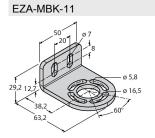
3071470 Mounting bracket, steel, blackfinished, for EZ-ARRAY and EZ-SCREEN standard and cascade 14 & 30 mm
