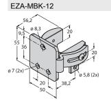
Mounting bracket, steel, blackfinished, for EZ-ARRAY and EZ-SCREEN standard and cascade 14 & 30 mm
