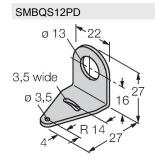
Mounting bracket; material VA 1.4401, for Q12 & M12 series
