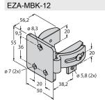
3071756 Mounting bracket, steel, blackfinished, for EZ-ARRAY and EZ-SCREEN standard and cascade 14 & 30 mm
