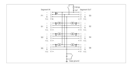
The 6-channel junction box JBBS-49SC-E613/3G is designed for FOUNDATION™ fieldbus systems.
