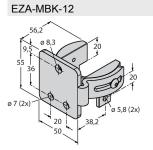
Mounting bracket, steel, blackfinished, for EZ-ARRAY and EZ-SCREEN standard and cascade 14 & 30 mm
