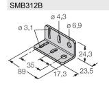
3025519 Mounting bracket, stainless steel, for MINI-BEAM NAMUR
