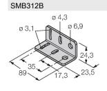
Mounting bracket, stainless steel, for MINI-BEAM NAMUR
