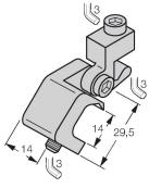
Mounting bracket for mounting magnetic field sensors on tie-rod cylinders; cylinder diameter 40... 125 mm; material: Aluminum
