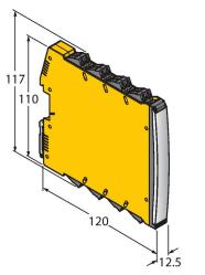
Isolating switching amplifier, 2-channel; SIL2 acc. to IEC 61508; Ex-proof version; 2 transistor outputs; input Namur signal; ON/OFF switchable monitoring of wire-break and short-circuit; toggle between NO/NC mode; signal doubling; removable screw terminals; 12.5 mm wide; 24 VDC power supply
