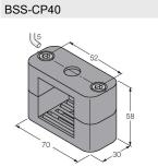
6901318 Mounting clamp for rectangular housings 40 x 40 mm; material: Polypropylene
