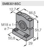
3053952 Mounting bracket, PTB black, for sensors with 18 mm thread
