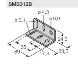
Mounting bracket, stainless steel, for MINI-BEAM NAMUR
