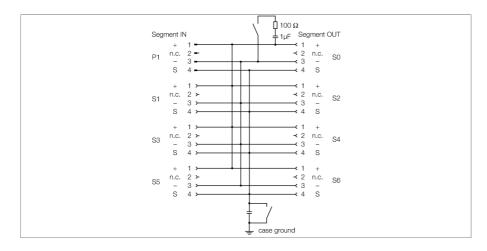
The 6-channel junction box JBBS-48-E613/3G is designed for PROFIBUS-PA systems.
