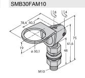
Mounting bracket, stainless steel, for M10 x 1.5 thread, thread length 30  $^{\rm mm}$
