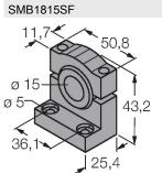
3053279 Mounting bracket, PBT black, for PICO-GUARD points SMB30A
