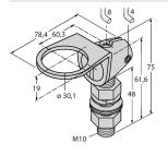
Mounting bracket, stainless steel, for M10 x 1.5 thread, thread length 30
