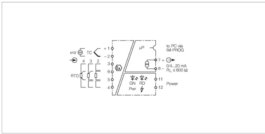
The temperature measuring amplifier IM34-11EX-CI/K70 is designed to evaluate the temperature-dependent changes of Ni100/Pt100 RTDs, thermocouples types B, E, J, K, L, N, R, S and T or low voltages in a range of -160...+160 mV and to output them as temperature-linear current signals.
