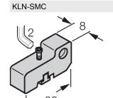
Mounting bracket for mounting magnetic field sensors on SMC cylinders; clamping width 4 mm; material: Anodized aluminum
