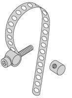
Mounting on round cylinders; cylinder diameter 8...25 mm; material: Metal CuZn; two tie bolts (material: Metal CuZn), cylinder screw M3 x 20
