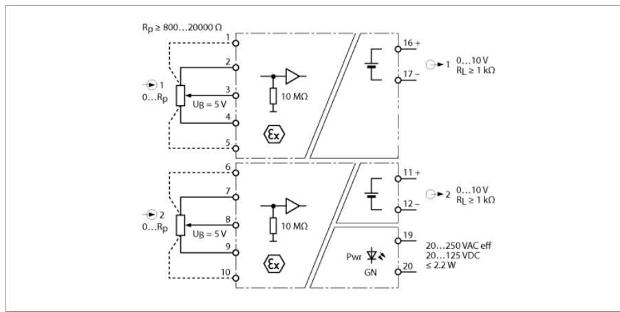
The 2-channel potentiometer amplifier IM36-22EX-U is designed to transmit signals from 3 or 5-wire potentiometers galvanically isolated from the Ex area to the non-Ex area and to convert them into normalized 0...10 V analog signals. The resistance value of the wiper contact, ranging from 0  $\Omega$  to the nominal resistance value (final value) of the potentiometer, is detected and linearly processed.
