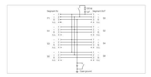
The 6-channel junction box JBBS-49-M613/3G is designed for FOUNDATION™ fieldbus systems.
