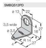
3059606 Mounting bracket; material VA 1.4401, for Q12 & M12 series
