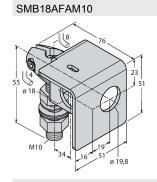
3012558 Mounting bracket, material VA 1.4401, for M10 x 1.5 thread, thread length 18 mm
