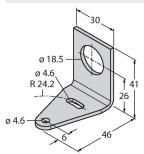
3012558 Mounting bracket, material VA 1.4401, for M10 x 1.5 thread, thread length 18 mm
