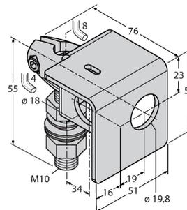
Mounting bracket, material VA 1.4401, for M10 x 1.5 thread, thread length 18 mm
