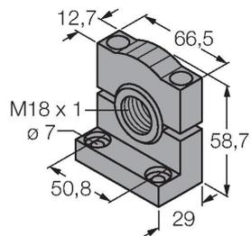
Mounting bracket, PTB black, for sensors with 18 mm thread
