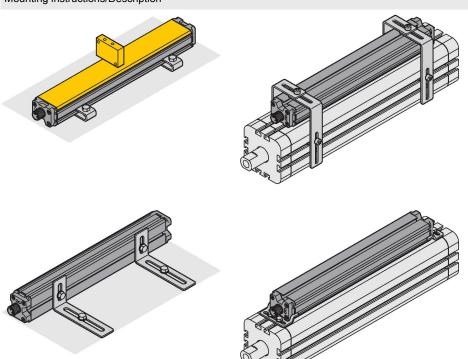
Numerous accessories allow the sensor to be mounted in various positions. Opposite to the active face, the sensor housing features a mounting groove for which sliding blocks are available. The lateral slot profiles can be used for mounting, too.
