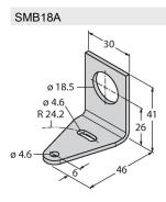
3033200 Mounting bracket, rectangular, stainless steel, for sensors with 18 mm thread SMB18AFAM10
