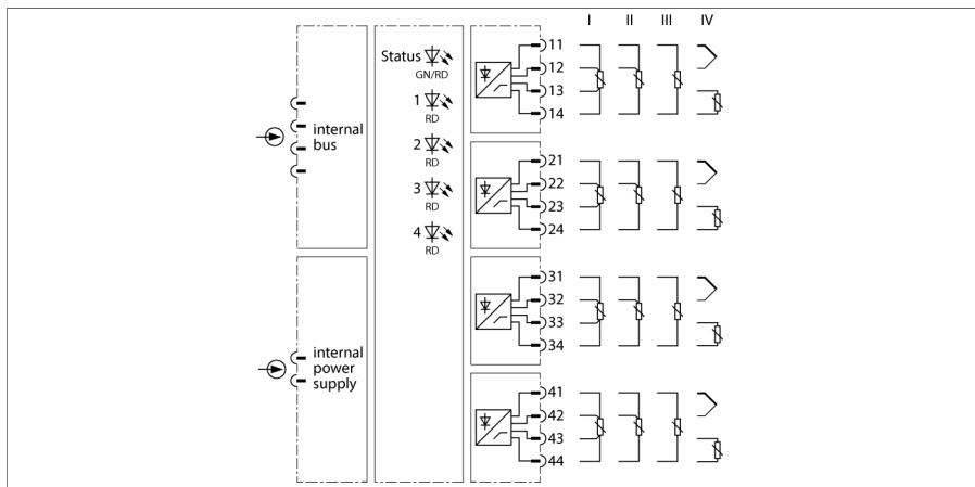
The input module TI40-N is used for the connection of 2, 3 and 4-wire temperature probes of the types Pt100, PT200, Pt500, Pt1000, Ni100 and CU100, as well as for the connection of thermocouples of the types B, E, D, J, K, L, N, R, S, T and U. The module can also be used for the measurement of low voltages (-75...+75 mV, -1.2...+1.2 V) and resistance measurements (0...30 Ω, 0...300 Ω, 0...3 kΩ).
