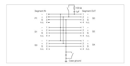
The 4-channel junction box JBBS-49-E413/3G is designed for FOUNDATION™ fieldbus systems.
