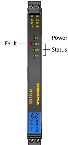
The IMX12-AI01-1I-1IU1R-H... isolating transducers are equipped with intrinsically safe input circuits and transfer analog measured signals from the Ex area to the non-Ex area. In addition, the devices monitor the input signals for exceeding or falling below an adjustable limit value. The devices are suitable for operation in Zone 2. Intrinsically safe (passive) 2-wire transducers, as well as active and passive HART transmitters, can be used on the devices in Ex areas.
