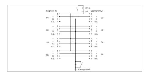
The 6-channel junction box JBBS-49-E613/3G is designed for FOUNDATION™ fieldbus systems.
