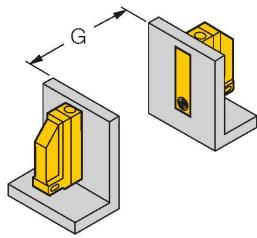
The sensors can be mounted directly side by side if a sensor with offset oscillation frequency Bi5U-Q12.../F2 is used.
