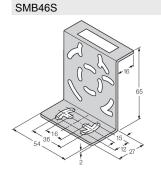
Mounting bracket, stainless steel, for QS18, QS30, MINI-BEAM, QM42/QMT42
