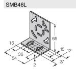
3048747 Mounting bracket, stainless steel, for QS18, QS30, MINI-BEAM, QM42/ QMT42
