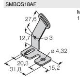
Mounting bracket, stainless steel, for 18 mm thread
