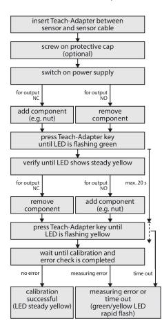
The measured signal in the sensor is influenced by the diameter and the material characteristics of the center bolt, but also by the cover of the sensitive area. Therefore each sensor has to be conditioned to the operating environment, i.e. to the applied sleeves or closure caps and the target (nut, sleeve etc.) To configure a sensor, the teach adaptor VB2-SP1 available from Turck is required.
