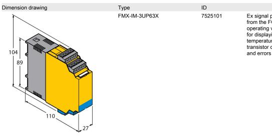
Ex signal processor for Ex flow sensors from the FC...-NAEX... product series; operating voltage 20...30 VDC; LED bar for displaying flow speed and medium temperature; IO-Link device with transistor outputs for flow, temperature and errors
