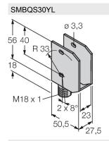
Protective housing with safety glas panel, stainless steel, for QS30 series
