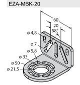
3072587 Mounting bracket, steel, blackfinished, for EZ-ARRAY and EZ-SCREEN standard 14 & 30 mm
