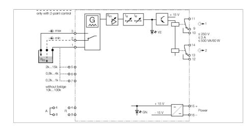
The 1-channel level controller MK91-121-R/24VDC monitors and regulates conductive liquid levels. As a dual level regulator, it can be used to control pumps amd solenoid valves, as monitoring device it is designed for run-dry or over flow protection
