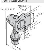
Mounting bracket, rotatable, stainless steel, for sensors of the Q4X/Q3X series, M10 x 1.5 thread
