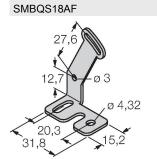
Mounting bracket, stainless steel, for 18 mm thread
